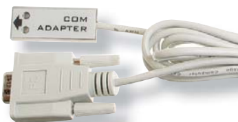
COM adapter for communication via RS232
